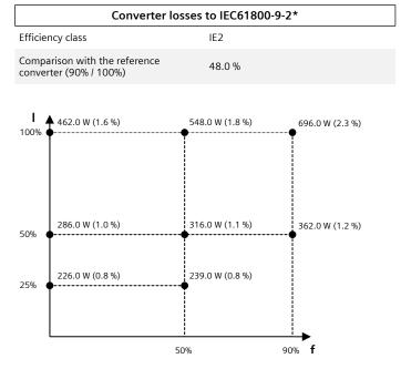
The percentage values show the losses in relation to the rated apparent power of the converter.
