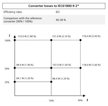
The percentage values show the losses in relation to the rated apparent power of the converter.
