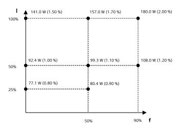
The percentage values show the losses in relation to the rated apparent power of the converter.
