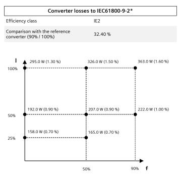
The percentage values show the losses in relation to the rated apparent power of the converter.
